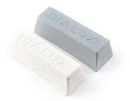
**DIALUX POLISHING PASTE** The gray one is for stainless steel and has a coarse grain. The white one is a finish for all kinds of metal. Aluminium oxide.  $20/32 \ \mu m$
